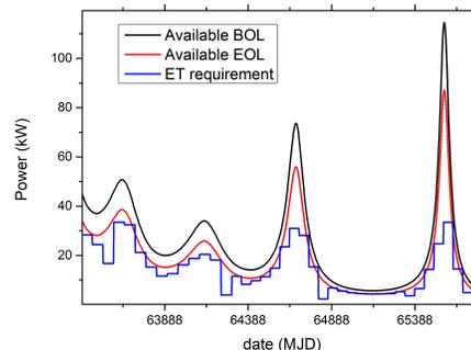
Figure 5: Power available as function of the time, for the BOL (black) and EOL (red) case. The power required by the space is plotted in blue.
