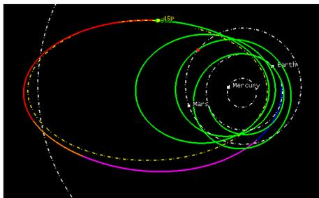
Figure 6: The complete interplanetary trajectory projected on the ecliptic plane. In details: in green the outbound trajectory with a Mars gravity assist at the red dot, in red the operational phase around the comet, in orange the departing maneuver, in purple the inbound cruise and in blue the braking maneuver.
