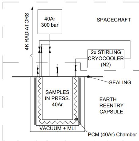
Figure 4: Scheme of the cryocooling system
