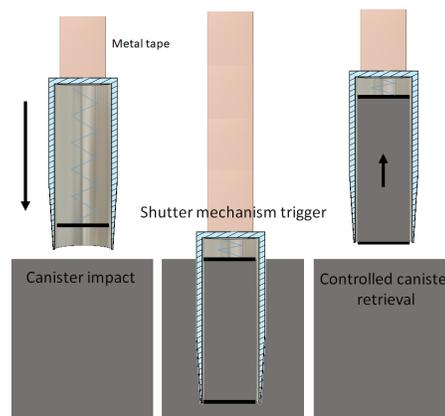
Figure 3: Sampling mechanism
