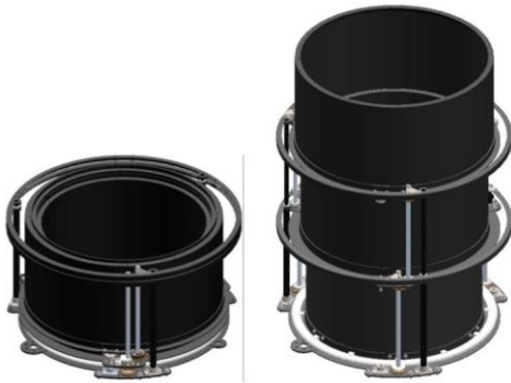
Fig. 1 Telescope structure in stowed and deployed configuration
