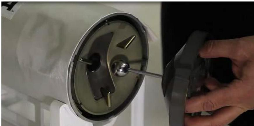
**Figure 4-13 - The MDA grapple fixture used on DARPA's Orbital Express Mission [65]**
