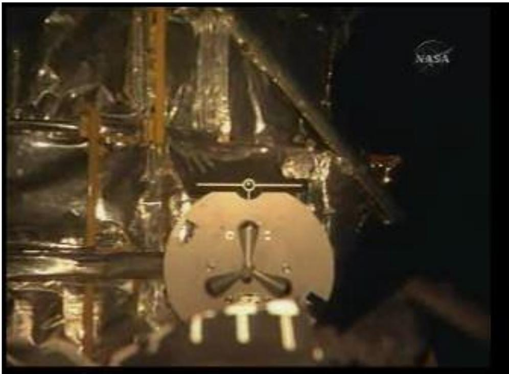
**Figure 4-7 - Hubble Space Telescope grapple fixture [126]**
