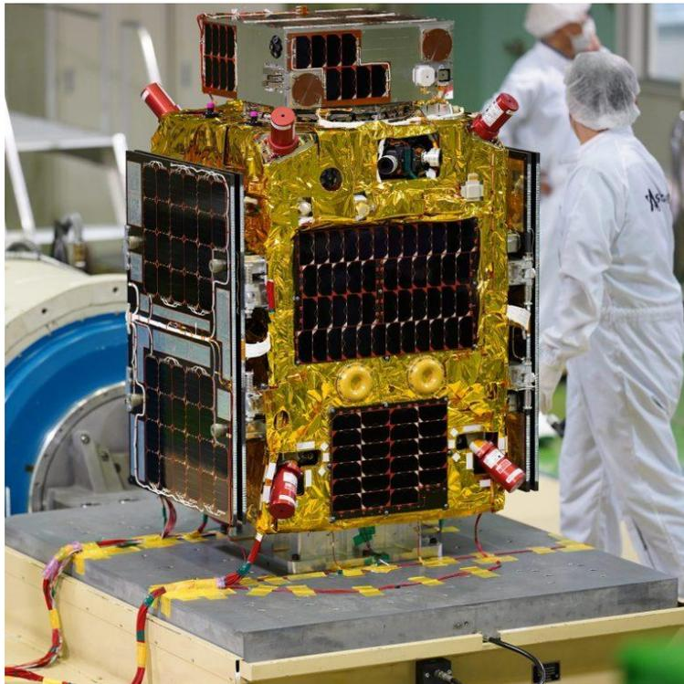
**Figure 4-4 - Astroscale ELSA-d spacecraft in a clean room [78]**
