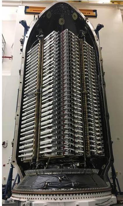
**Figure 5-3 - A stack of 60 Starlink satellites in their Falcon 9 launch vehicle's fairing prior to launch [158]**
