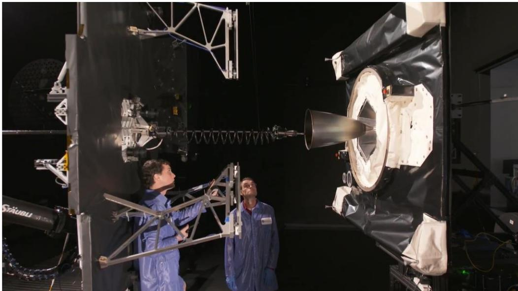
**Figure 4-14 - Testing of the MEV's probe attachment mechanism [147]**
