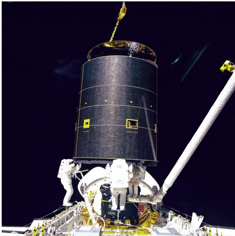
**Figure 4-2 - Intelsat VI being captured by three crew of STS-49 [54]**
